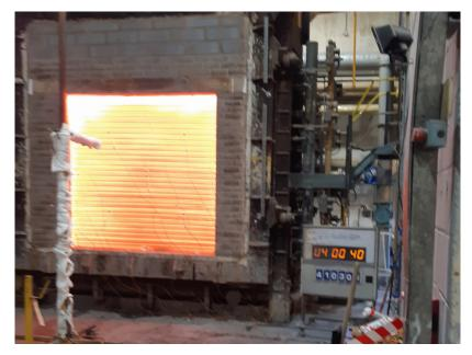
Our safe and reliable fire shutters are fully tested and certified in accordance with the latest fire standards BS EN 1634 -1:2014 + A1:2018 & BS EN 16034:2014.
